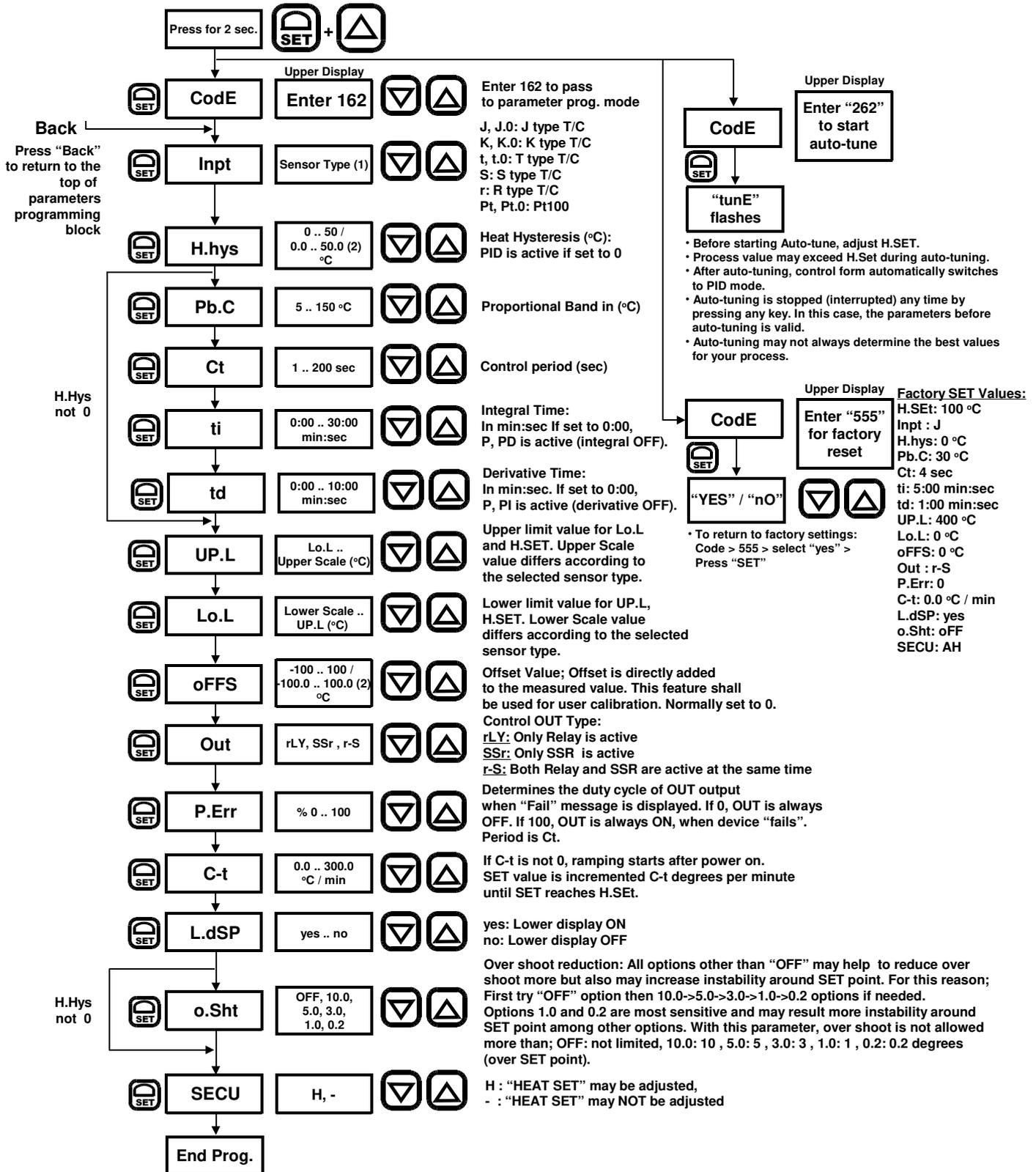
(1) When sensor type is changed, Up.L, Lo.L, H.Set, H.hys, oFFs may be set to a new value automatically, according to the selected sensor.
